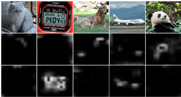
Figure 1: Visualization of various kinds of images (first row) along with the feature map of the 5-th and 144-th channel (second and third row, respectively) in the conv12 layer of VGG16-Net trained on ImageNet. (Best viewd with zooming in) All feature maps are with their origin activation value and size.
